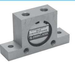
Ball vibrator could be used for bulk material release if the bulk material was adhesed on walls of tubes or filling hopper. It can be used for such as materials which doesn't solidify by intensive shedding; in this case pneumatic knocker should be used.
