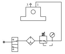
There is useful to use pressure regulator in circuit to enable vibration intensity regulation. If you need to start vibrator by another way than manually, there is necessary to use appropriate 2/2 or 3/2 valve which should be connected between pressure regulator and vibrator.
