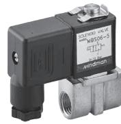
Direct solenoid actuated valve 2/2 normally closed with orifice 1 to 2.4 mm. The following sealing are available: NBR, EPDM and viton (teflon on request). Available fluid: air, inert gas, water, vacuum, oil, etc. Coil with Ex approval EExm II T4, or EEx ia II C T6 PTB are available on request.
