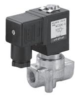
Direct solenoid actuated valve 2/2 normally closed with orifice up to 4 mm, as extension of series MBS. The following sealing are available: NBR, EPDM and viton (teflon and other on request). Available fluid: air, inert gas, water, vacuum, oil, etc. Coil with Ex approval EExm II T4, or EEx ia II C T6 PTB are available on request.
