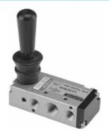
Valves are available with or without detent as well as functions 5/2 and 5/3 with closed, pressured or exhausted centre. Valves can be mounted by using the holes on the valve body, type MVHB 220 can be also mounted into the panel with hole dia. 18.5 mm.
