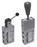
Lever valves are actuated by 120° lever turning. Both positions are detent. Draw bar valves are actuated by pressing the draw bar. Return to starting position is by pulling of draw bar. If the draw bar is during pulling out rotated to right, the force which is need for overcome the detent will be lower. Draw bar valves can be produced from stainless steel on request.
