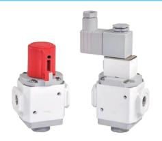
Shutoff valve is an easy and inexpensive way to add shutoff capability to an FRL unit. It allows the air supply to be closed and MVHR models can be operated either manually or by a solenoid valve. When the supply is closed, the compressed air is exhausted from the circuit behind the valve. Both positions of the manually operated model can be locked (padlock not included), which will contribute to safety during maintenance or adjustment. The valve is designed to be assembled
