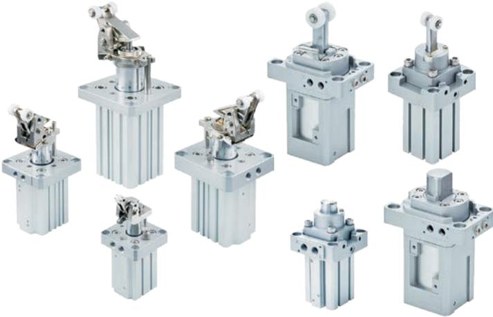
Stopper cylinders are used for safety stop or separation of objects which moves on belt, roller, chain or other conveyor. Regarding the series (see description below), the cylinders can be equipped for example with hydraulic shock absorber for soft stop of moving object, or with spring for automatic separation of two objects.
