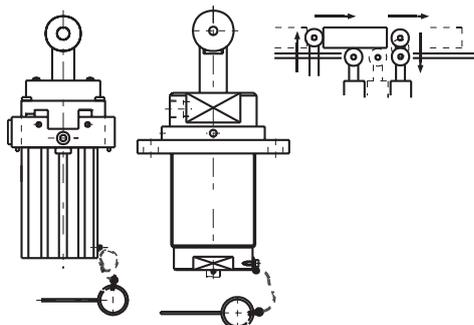
The top rollers with the built-in spring return in touch with the bottom of the work carrier. Automatically returns up to the original position as the work carrier pass by, and immediately works as a stopper for the next work carrier. Therefore the timing carriers does not need to be taken.
