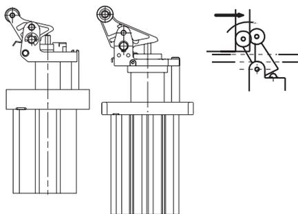
The built-in shock absorber softly catches and stops the work carrier. The strength of absorber can be easily adjusted, which makes the cylinder work in the best condition, conforming to the speed of the conveyor line and the weight of the work carrier.
