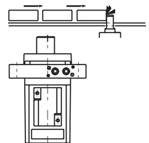
Rod and cylinder are designed for toughness against the large side load. Also suitable for the relatively slow-moving conveyor line with the heavy work carriers.
